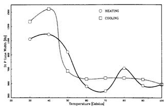
Figure 3. 31P MAS line width of PBFP during heating and cooling after annealing at 200 °C.
